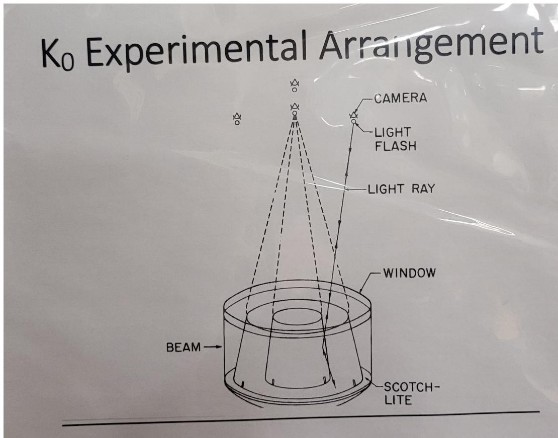
Above is a diagram of the set up of a bubble chamber.
